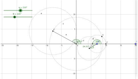
For example, as the above figure, if the angle CAE' is  $151.2^{\circ}$ , then we don't have a connected linkage. Hence with certain angles like this example, we don't have a connected linkage—which means we can't use an  $S^1$  to glue all copies. And so, if we fix the shorter one (with length 3), then in each angle, we still can have a validated linkage that move in certain range of angles. (This will be proved in the next section.)
