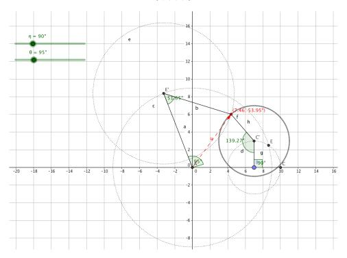
Theoretically, each movement can be validated by using triangle inequality, but it's handy to check this just directly using a GeoGebra model to see the linkage moving in action continuously. A snapshot of this experiment is in the above figure.
